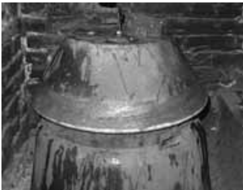
図2-12 粘土で淵を閉じた釜
